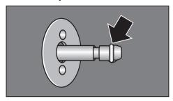
A connector between the brew unit and coffee dispenser is located on the inner door.
